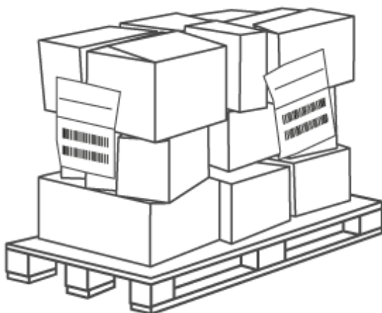
Figure 4 Irregularly packed pallet.
